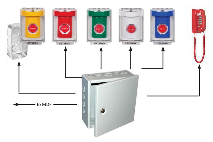
The Campus Notification System is a grouping of notification devices including the fire voice evacuation public address panel, the area of refuge panel if needed, an analog wall mounted red phone and Campus Notification Panel with buttons for initiating emergency notification broadcasts to the campus. All of these systems should be located in the same area of the main office and be easily accessible by School Staff.
